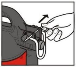
Pull the safety pin to unlock the lever
