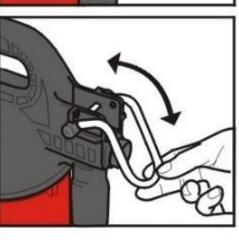
• Then, **pull** the lever upwards to pressurize.
